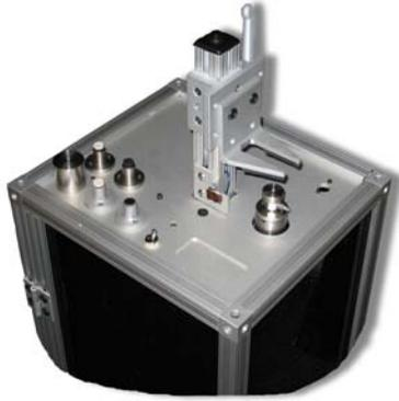
Figure 3: 9155C-525 pneumatic shock exciter
