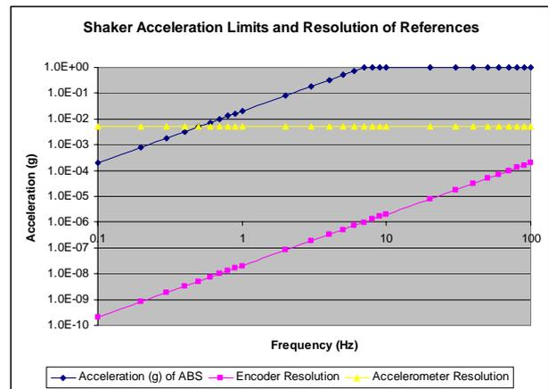
Fig. 5. Theoretical limits of accelerometer\* and optical encoder reference sensors charted against air-bearing shaker acceleration limits due to maximum stroke. \*Accelerometer resolution displayed is based upon the manufacturer's broadband RMS resolution of the air-bearing shaker's integral reference accelerometer.
