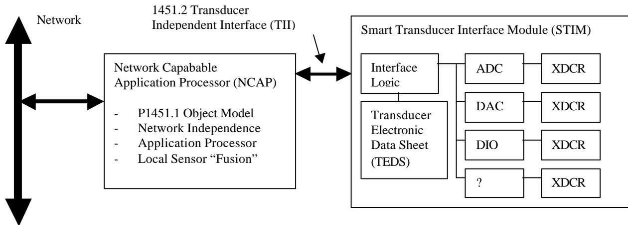
Figure 2 – System block diagram showing a 1451.1 and 1451.2 interface to an integrated STIM
