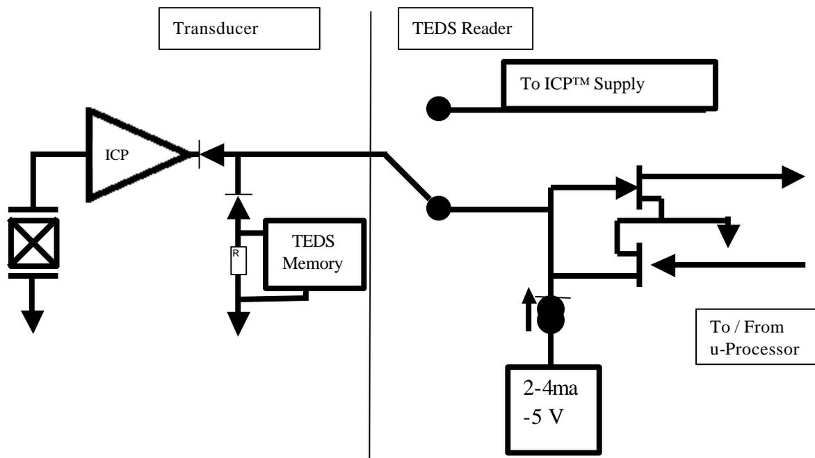
Figure 4 Example of a two wire constant current ICP™ 1451.4 implementation
