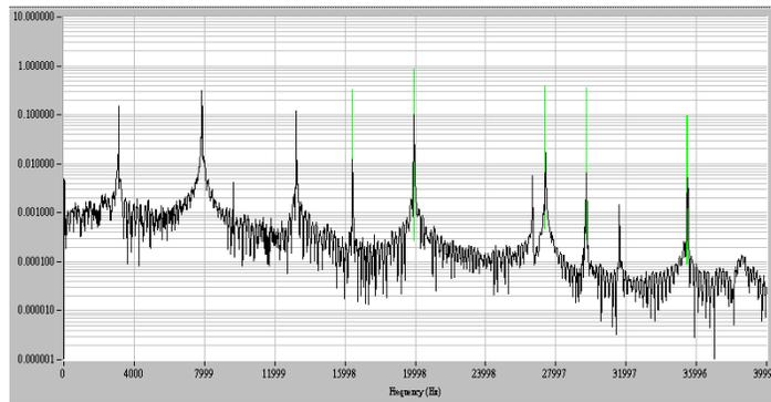
Figure 2. Typical acoustic signature for powdered metal part.
