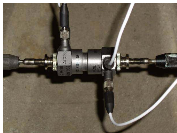
Figure 7 -- Close up of impedance head installation
