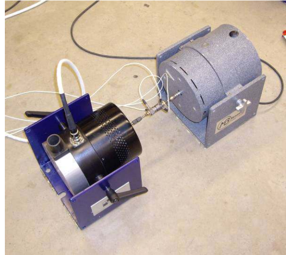
Figure-4 -- Back-to-Back Configuration with MB-50 (50lbf) and 2100E11 (100lbf) exciters hot glued to floor
