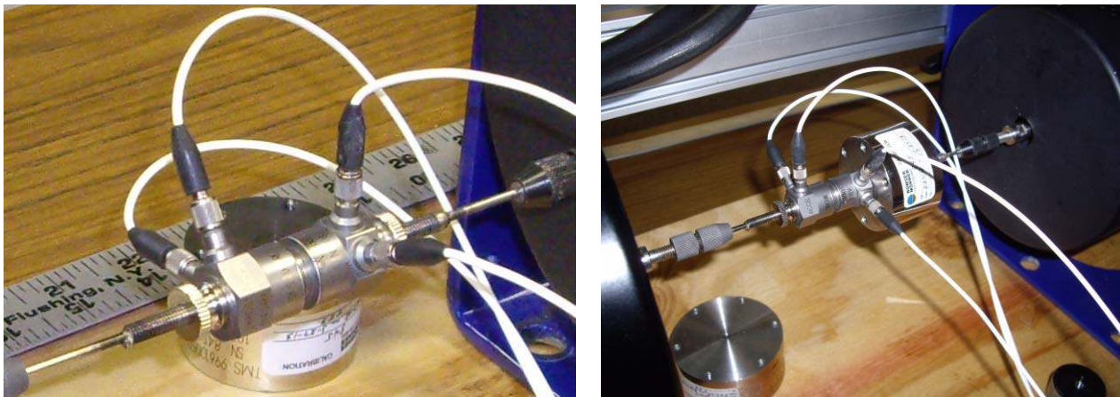
Figure 10 -- Pictures of the B2B Impedance Heads no-mass and mass additive configurations.
