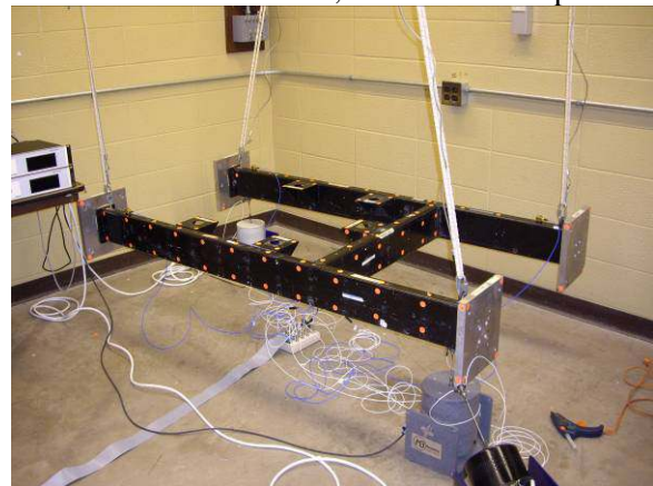
Figure 5 – H-Frame MIMO Test Setup
