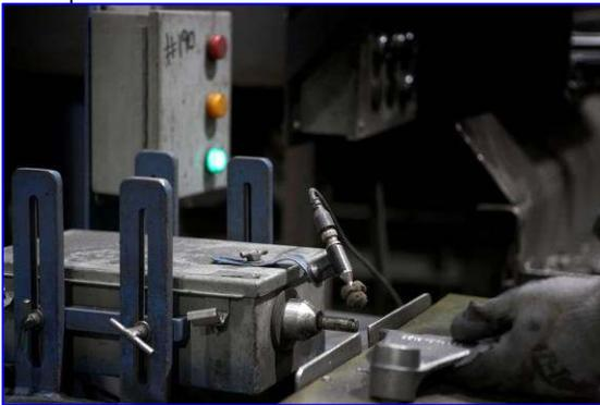
Durability of the test system was also key for Urick. From the rugged microphone and industrial electric impactor to the NEMA4 packaged smart digital controller, the RAM NDT design excels in industrial environments. Its durable, physical construction is perfect for plant floor, high volume, test applications.
