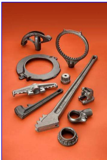
machines. The properties of ductile iron make the pouring of castings a bit tricky. The inoculation of the molten iron with magnesium creates the possibility of nodularity “fading” if the castings are not poured quickly. Urick uses a delayed in-mold technique, which minimizes the variations that affect product quality.
