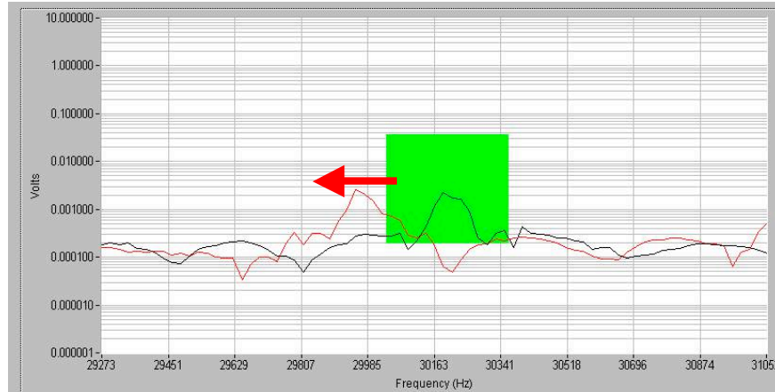
Figure 3. Data showing a typical frequency shift detected by NDT-RAM.
