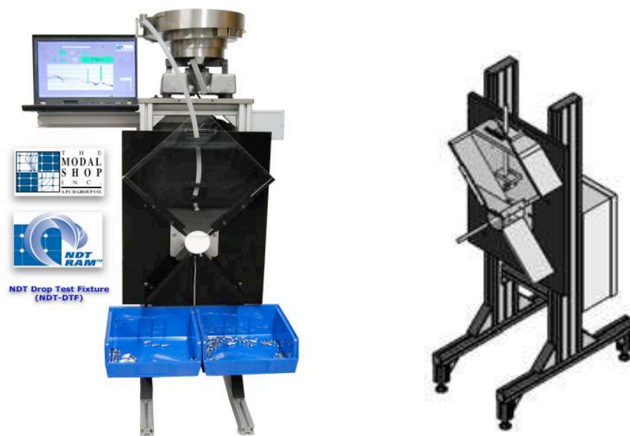
Figure 5. NDT-DTF Drop Test Fixture with LanSharC data processor and laptop controller.
