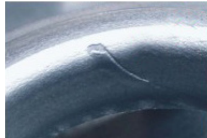
Crack formed during drawing process
