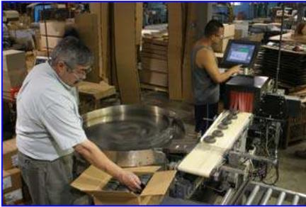
“We’ve incorporated the RAM NDT unit right on our assembly line,” says Rich Slattery. “It doesn’t slow our production one bit. Components pass through it right before packaging. Any product that doesn’t pass inspection is removed from the line automatically. And gears that pass inspection are immediately packaged and shipped in a streamlined operation.”
