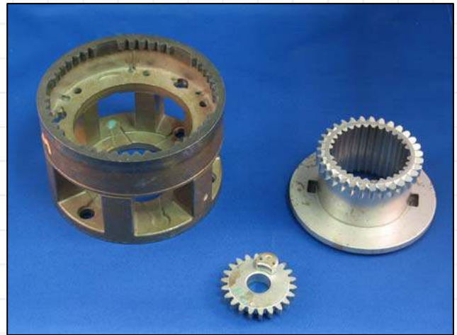
Fig 1. Sinter braze powder metal components
