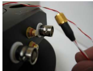
B) Carefully disconnect the insert's signal cable.
