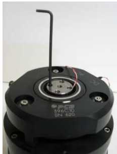
A) Remove the screws with supplied hex wrench.
