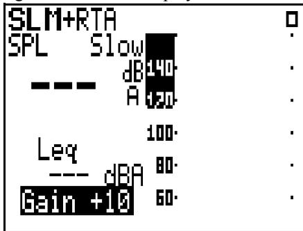
When the gain setting is highlighted, this can be changed by repeatedly pressing the ▲ or ▼ key until the desired value of Gain appears.
