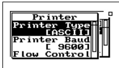
*Depending on your printer configuration you may have to modify the Printer Settings for Printer Baud Rate and Flow Control.*
