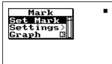
*When “Set Mark” is initiated by pressing the Check (✓) key, a marker is placed into the time history record at that point in time.*
