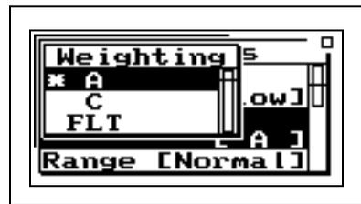
**Step 5** Highlight the desired weighting and press the  $\checkmark$  Check key.
