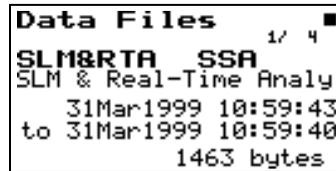
*The **Data Files** screen shows the currently selected record number, the ID used to take the measurement, the start/stop dates and times, and the total bytes used by the record.*
