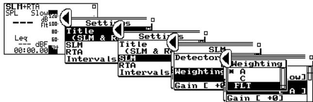
In this particular instance, when the **▶** key was used to move from the Settings menu to the SLM sub-menu and from the SLM sub-menu to the Selections menu, the item highlighted was not the first in the list. Observe that when **Ⓢ** was pressed to accept the selection of “FLT for the frequency weighting, upon returning to the Weighting sub-menu, the 2nd item was highlighted, just as it had been previous to entering the Selection menu using **▶** .
