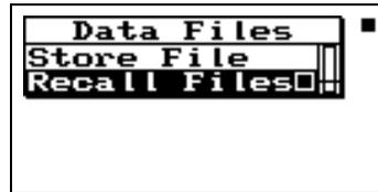
*When recalling a data file, the System 824 will automatically switch to the instrument that the data file was stored as (i.e. from Logging to SLM&RTA).*
