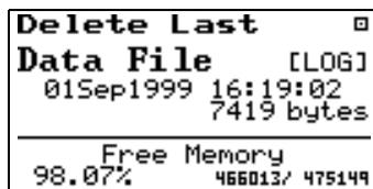
This display shows the last record that was stored along with the date and time of the data, the instrument type it is
