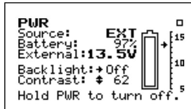
This simple display indicates that the System 824 is plugged into an external source which is 13.5 volts; the battery is 97% full; the backlight is off; and contrast is at 62%.
