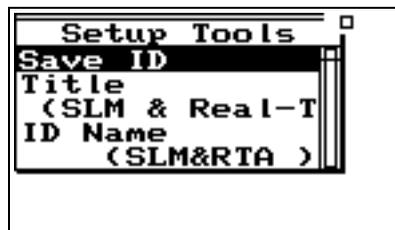
With the **Setup Tools** menu you can create and/or modify instrument definition (ID) settings. The **Setup Tools** menu provides the following three options, which are later described in greater detail.
