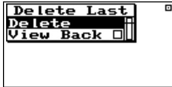
**Step 5** Highlight "Delete" and press the Check (✓) key. The record is deleted. If the last record was a data file then the following choices will appear:
