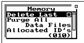
**Step 4** Highlight “Delete Last” and press the Check
