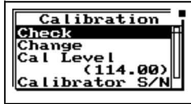
**Step 9** Place the calibrator over the microphone, switch the calibrator ON, and press  $\checkmark$  to activate the calibration **Check** process.
