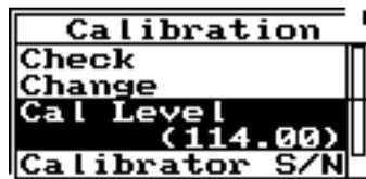
*NOTE: The output level specified by the calibrator manufacturer will be at standard temperature and pressure. In practice the level is a function of temperature and static (barometric) pressure, so a corrected level should be used. Similarly, the sensitivity of the microphone itself is a function of temperature and static pressure. For directions on compensating for temperature and static pressure during calibration, see "Correction of Calibrator Output Level" on page 2-17.*
