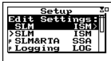
At any time, one of the available setups will be the active setup. The name of this setup will be at the top of the list below the Edit Setting message. Pressing the
