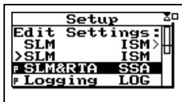
**Step 1** With SLM&RTA highlighted, press **▼** to select it as the current ID.
