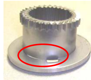
Figure 5. Gross misalignment defect (indicated by gap within red circle) common with sinter brazed powdered metal parts.
