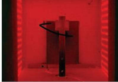
This shows a 1,200 F accelerometer under test. Note that under these conditions a functioning accelerometer is actually glowing. Source: PCB
