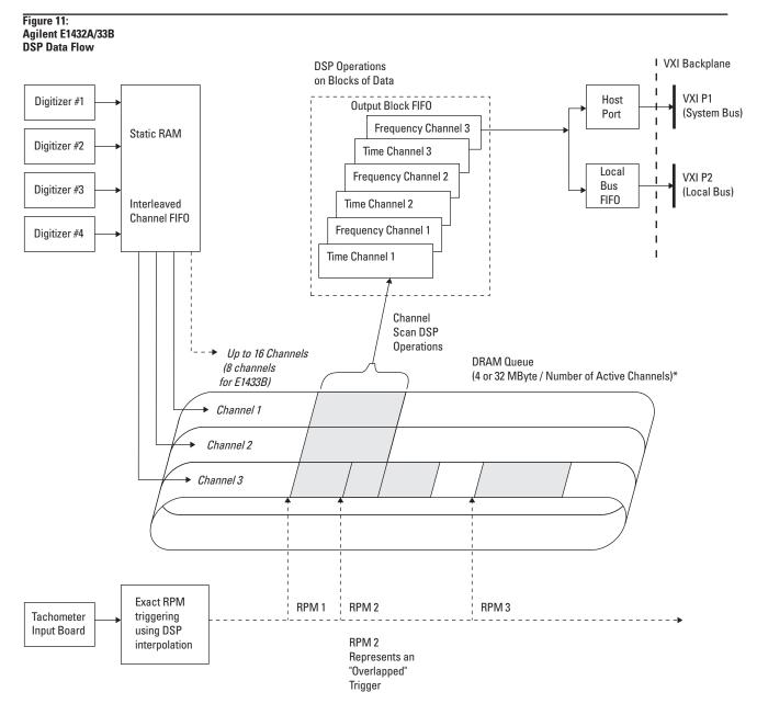
\* Note: FIFO size reduced with octave and peak/RMS calculations.
