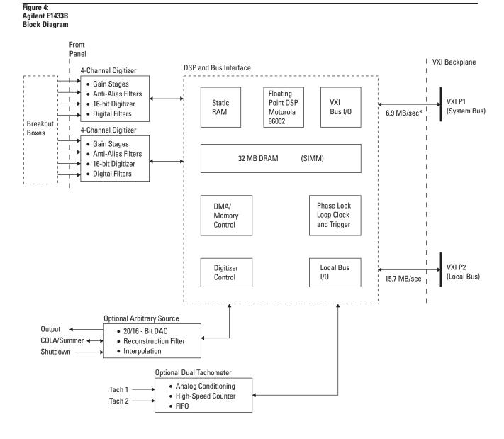
\* 6.9 MBytes/sec represents the transfer rate over the VME bus when sending the 16 bit integer samples from the ADC to the host. A more typical transfer mechanism would be using the readFloat64Data which stores the data in the host as 64 bit floating point values. In this case the transfer rate is 27.6 MB/sec considering the 64 bit format as stored in the host.
