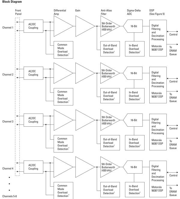
Figure 2: Agilent E1433B **4-Channel Digitizer**
