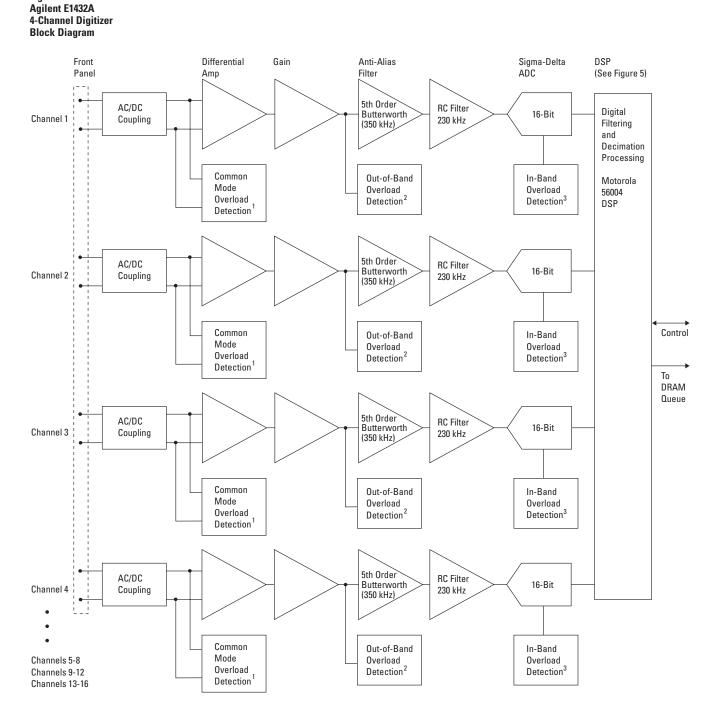
1 Detects common mode overloads in differential amplifier.
