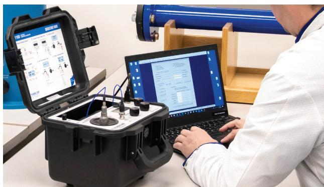
The Portable Vibration Calibrator Model C9110D-T was designed for use in energy, industrial, and military depot calibration environments. As the heart of the 9140 Series, the C9110D-T is a reliable and precision device proven to serve as a work horse in any vibration calibration program.
