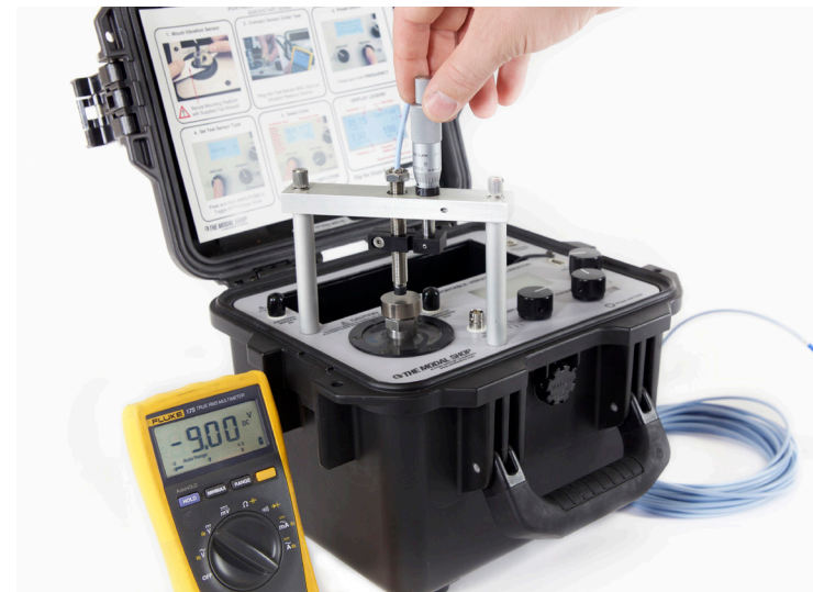
Technician adjusts position of proximity probe to correct for this error
