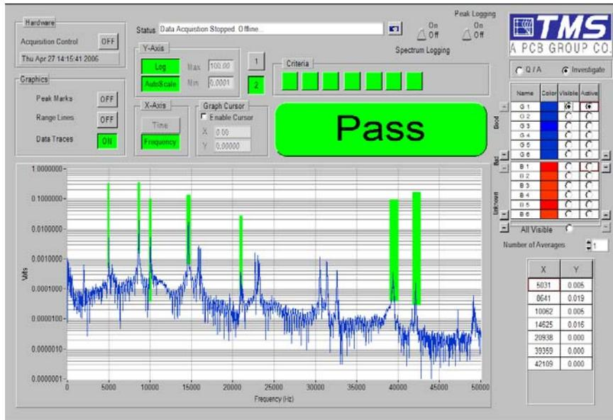
**Figure 2.** Typical acoustic signature, power spectrum to 50 kHz, for a metal part, shown as processed by NDT-RAM with criteria ranges (indicated with green “boxes”) at seven natural resonant frequencies.
