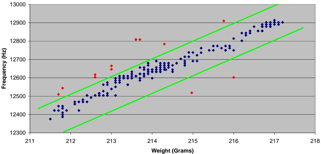
**Figure 11.** Skewed criteria limits set using ARAM about the 12,500 Hz resonance
