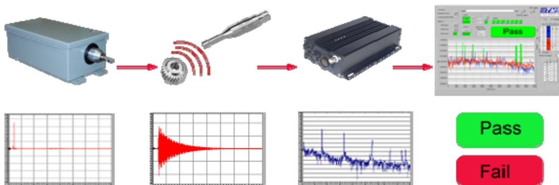
**Figure 1.** NDT-RAM process flow.
