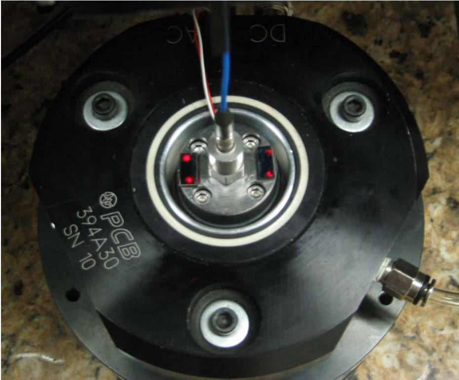
Figure 3. Top view of The Modal Shop 394A30 air bearing shaker, showing implementation of dual beam multi-pass laser for primary vibration calibration.
