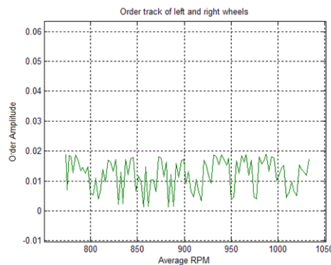
Figure 4: Zoom in of order track, theoretical amplitude = 0.01.
