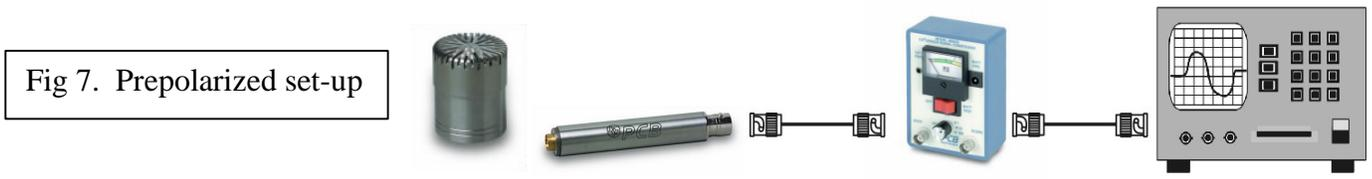
Components of the prepolarized design may be used with the externally polarized set-up. The prepolarized microphone can be used with a Power Supply that is designed for externally powered microphones, and its associated preamp, provided that you set the supply voltage to zero.
