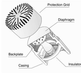
Fig 1. Microphone Components
