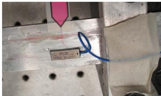
Fig. 1. Aluminium cantilever beam with FBG and ICP sensors
