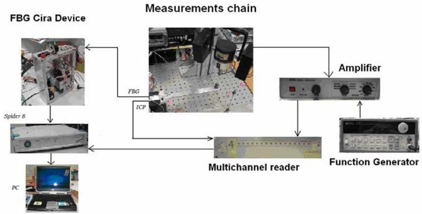
Fig. 2. Measurement System Block Diagram
