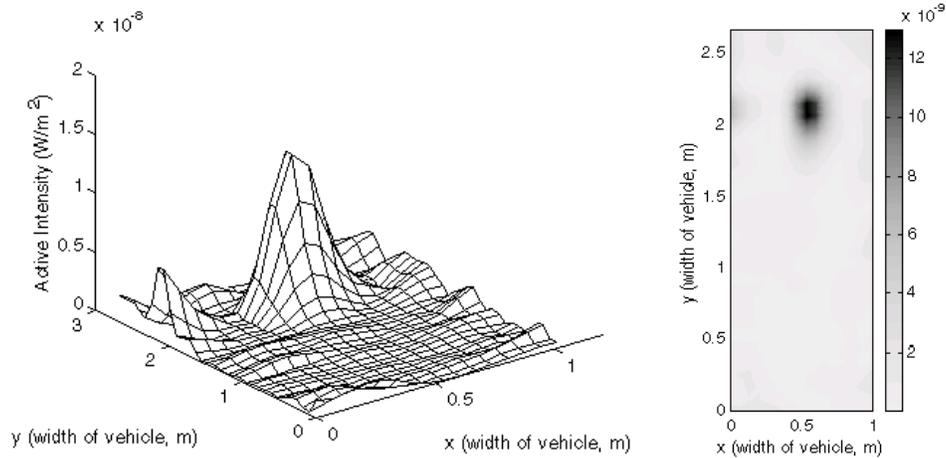
Figure 9: **3-d mesh and gray-scale map of the reactive intensity projected onto the floor pan.**
