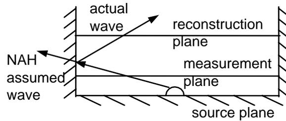
Figure 3: **Illustration of a wall reflection.**
