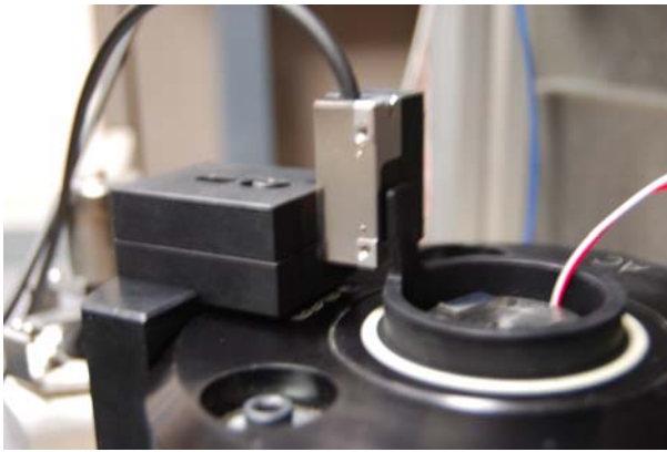
Fig. 6. Optical encoder read-head sensor and read-strip optical scale mounted on Model 394A30 calibration air-bearing shaker.
