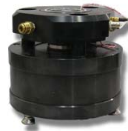
Fig. 3. Precision air-bearing calibration shaker
