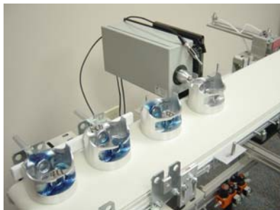
Figure 5. Industrial electric impact hammer designed for millions of impacts and rugged microphone for non-contact response measurement, shown mounted on conveyor section.
