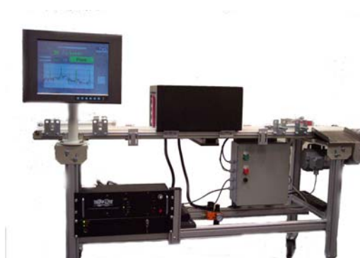
Figure 7. Fully automated system on 6 ft conveyor section, shown with acoustic chamber for testing parts.
