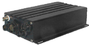
Figure 6. Smart digital controller measures signals and processes data, independent of PC, with internal digital relay outputs.
