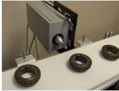
Figure 5. Industrial electric impact hammer designed for millions of impacts and rugged microphone for non-contact response measurement, shown mounted on conveyor section.
