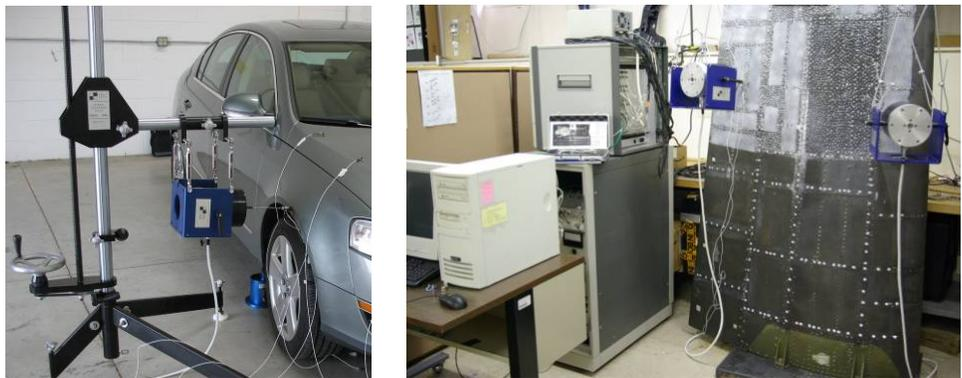
Figure 3 – Typical shaker excitation setup
