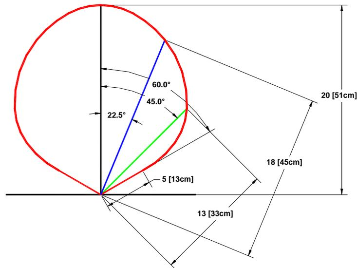
**Figure 6 – Typical Operating Envelope For LaserTach**
