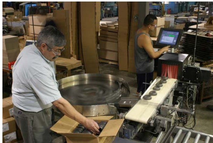
Figure 3. Fully automated system on plant floor, shown testing parts through acoustic chamber.
