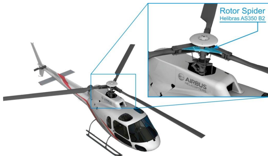
Figure 1: Helicopter AS350 from Eurocopter - rotor spider location (based on image taken from http://www.airbushelicopters.com/ )
